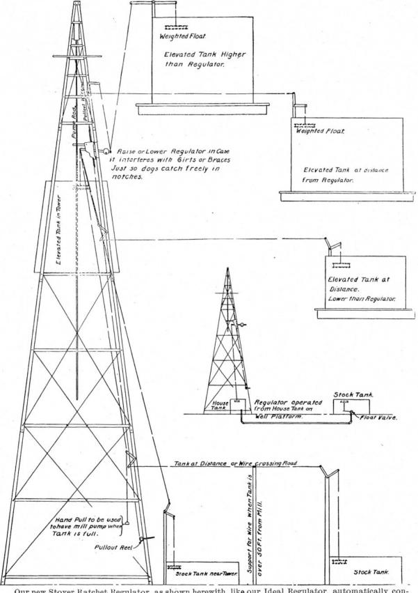
Our new Stover Ratchet Regulator, as shown herewith, like our Ideal Regulator, automatically controls the Wind Mill and Tank supply. Unlike the Ideal, it is fastened high in the Tower, as shown in sketch and clamps to any one of the corner posts on 3 or 4-post steel Towers and wood Towers. With our Ratchet Regulator it is possible to set the Tank at any angle from the Wind Mill Tower.
