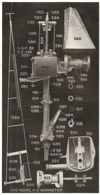
The above shows the parts of the Auto-Oiled Aermotor of the 1916 Model. Repairs for the different sizes are designated by the letter "X" for 6-foot, "A" for 8-foot mill, "B" for 10-foot, "D" for 12-foot, "E" for 14-foot and "F" for 16-foot.
