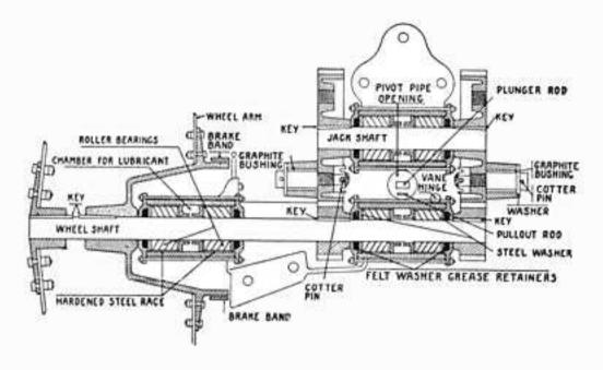
THESE roller bearings take the place of babbitt bearings on the shafts, and thus eliminate practically all the friction.
